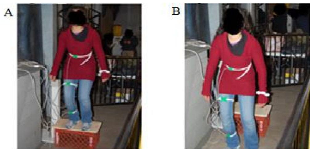
Figure 4.3 (A) One participant while jumping off of the 30 cm block, (B) Subject upon landing. The location of each of the three trackSTAR sensors is included.
