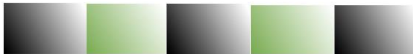
Figure 4.1 Desired theoretical nanoheterostructure, where black represents boron and green represents boron nitride. This could be a nanowire or nanotube heterostructure.
