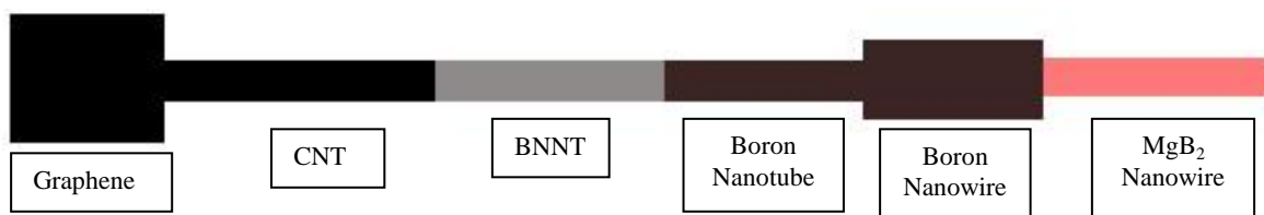
Figure 7.2 Nanowire of sections of material which could be created through the IL method. Graphene could easily be joined with CNTs.
