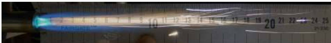
Figure D.1 Rotated photograph of air-acetylene flame with seeded Al-wax powders. Flame conditions were the same as for Al-cyclooctane in Chapter 6.
