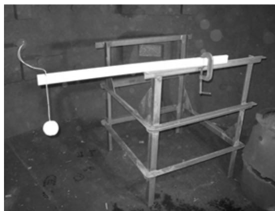
Figure 5.10 Blast test setup for quantitative blast tests; gage ports visible behind frame.
