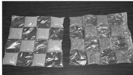
Figure 1.3 Quilted bentonite jacket, with “checkerboard” fill pattern.
