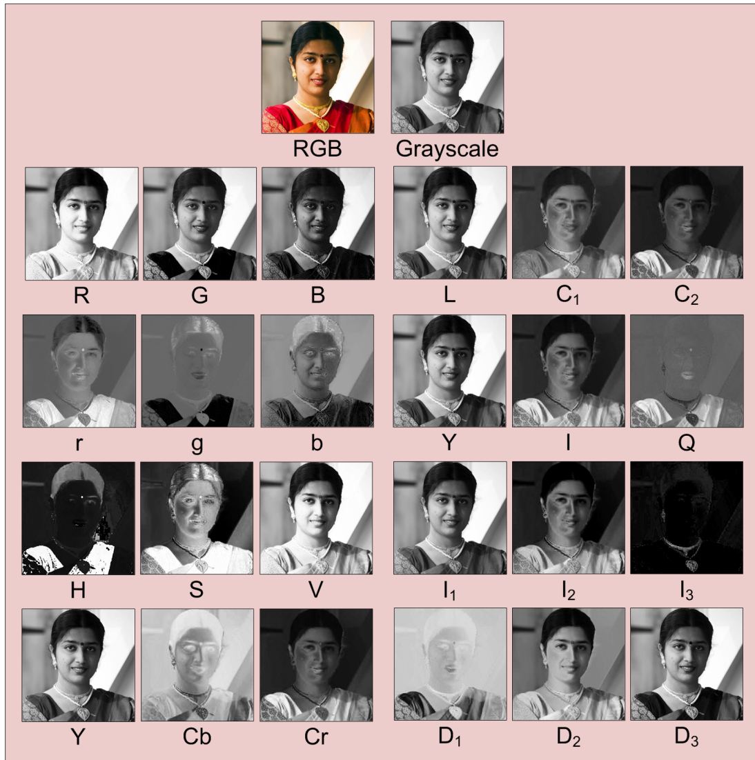
Figure 2.1 An RGB color image, its grayscale image, and the color component images in the RGB, oRGB, rgb, YIQ, HSV, I_1I_2I_3 , YCbCr and DCS color spaces, respectively.
