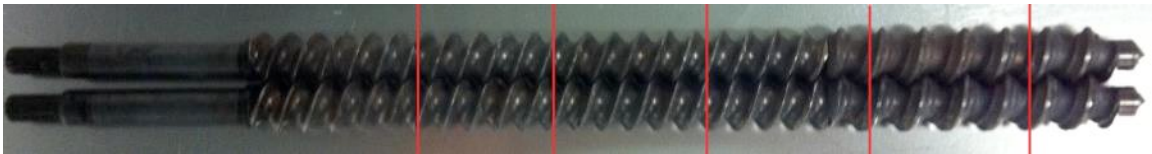
Figure 4.38 Screws used to investigate the effect of particle size on the dissolution process of API (CS).
