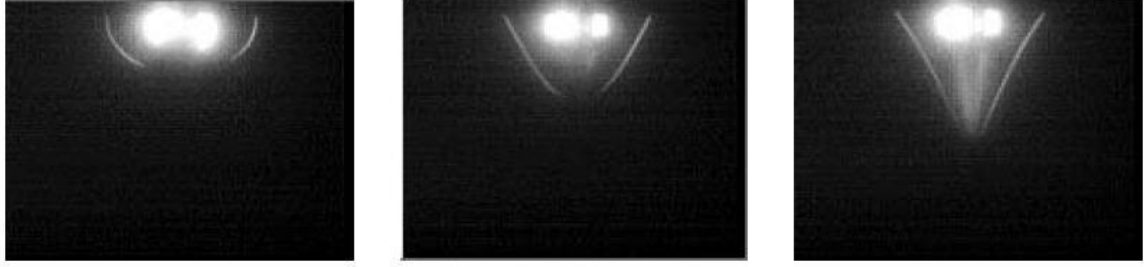
Figure 1.3 Formation of the Taylor cone. Voltage increases with each stage until equilibrium between surface tension and the electrostatic force is approaching to the limit [18].
