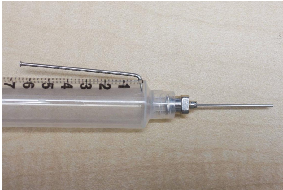
Figure 2.7 Modified syringe assembly used for electrospinning process.
