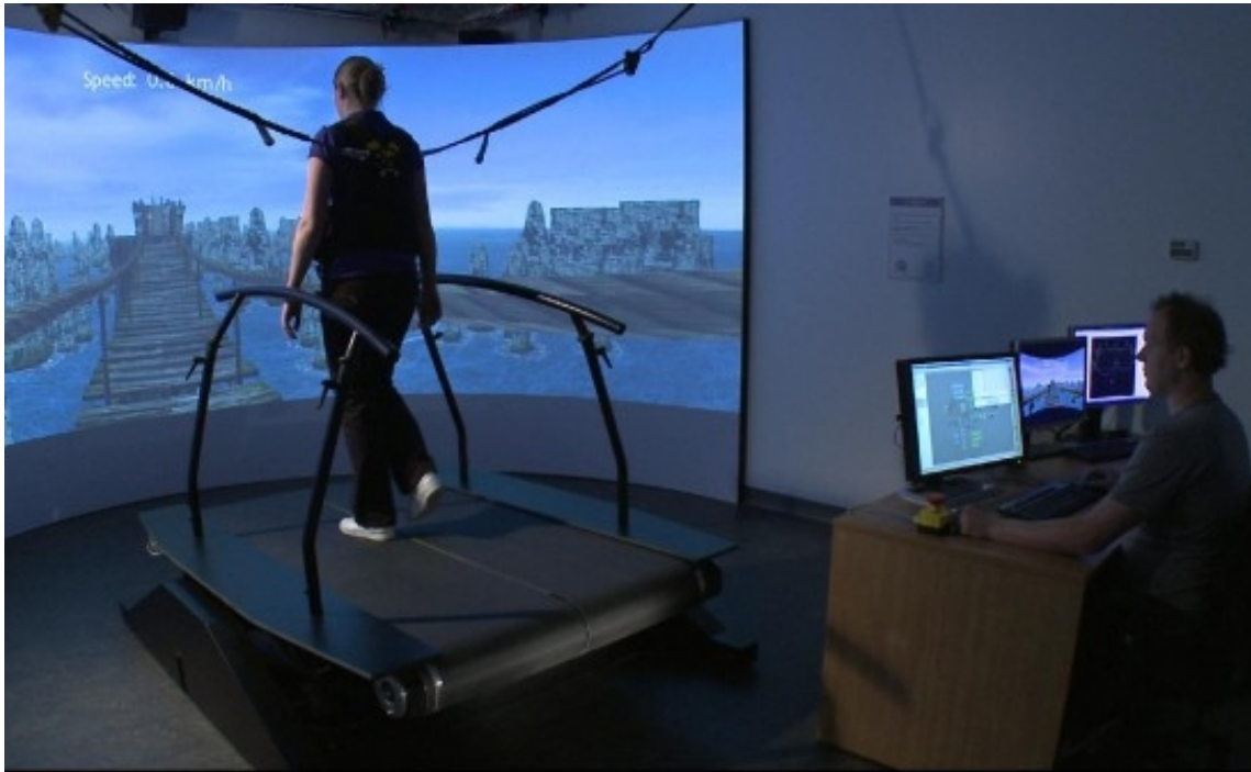
Figure 1.2: Motek's virtual environment with assistive treadmill for gait training.
