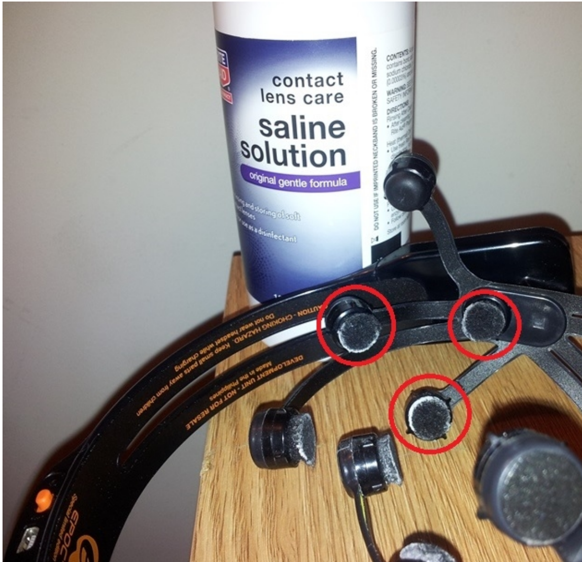
Figure 5.1: Emotiv EPOC Headset, felt sensors highlighted in red with the saline solution. The white patch on the felt sensors is due to the deposited salt and needs to be washed off or changes after extensive usage.
