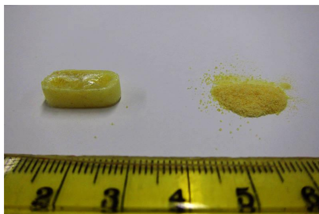
Figure 4.12 Volume difference between the foamed pill and the amount of powder used before batch foaming process.
