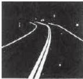
Figure 2.3 (a) Pavement markings with reflective beads.
