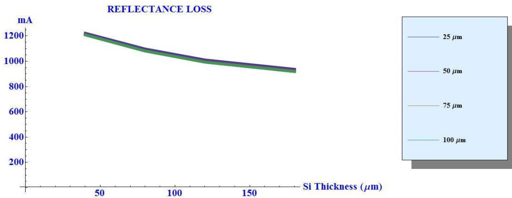
Figure 5.10 Plot of reflectance loss values for module with respect to silicon thickness for metal finger width of (a) 100 \mu\text{m} , (b) 75 \mu\text{m} , (c) 50 \mu\text{m} , and (d) 25 \mu\text{m} .
