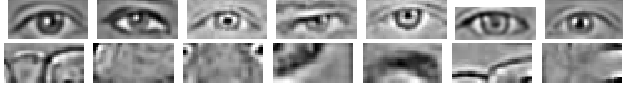
Figure 3.4 Example eye (the top row) and non-eye (the bottom row) training images that are normalized to 20 \times 40 . The images are preprocessed by illumination normalization.
