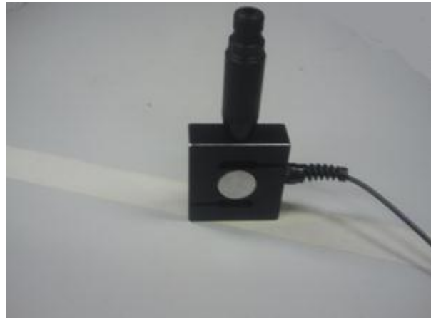
Figure 3.2 Strain gage with installed handle to simulate sonography probe.
