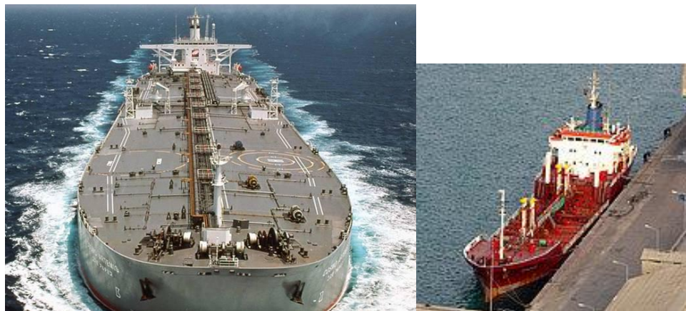
Figure 4.2 Tankers. Very Large Crude Carrier (left), Small Wine Tanker (right).
