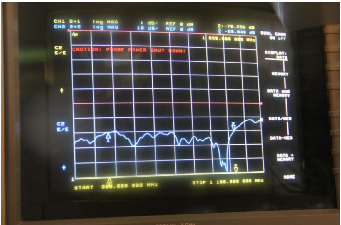
Figure 4.17 Return loss test results for RFID antenna.
