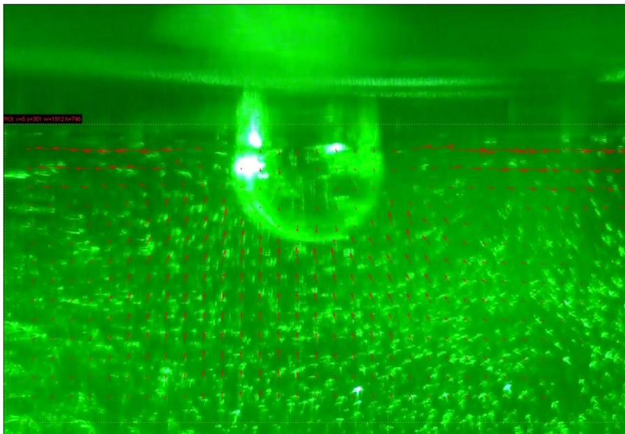
g) t = 0.55 s. The flow pattern is qualitatively similar to the previous photograph. The average velocity of the field is 0.977 mm/s.
