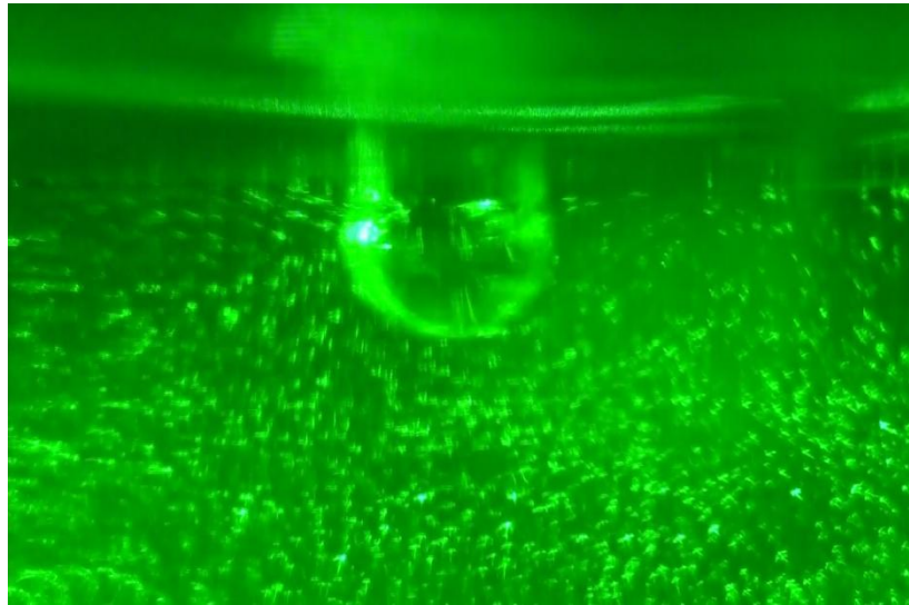
Figure 6.3 Velocity distribution 0.3 s after a test particle touches the interface. The figure shows the seeded particles and the air water interface.
