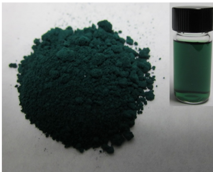
Figure 3.6 PANi-PSSA powders with its solution in water after two months.
