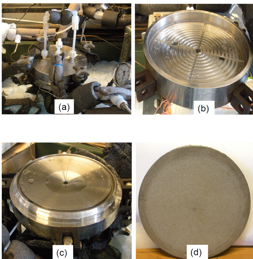
Figure 3.26 Photographs of (a) large cell used for experiments (b) top of the cell (c) bottom of cell (d) 6 mm thick stainless steel support for the membrane.
