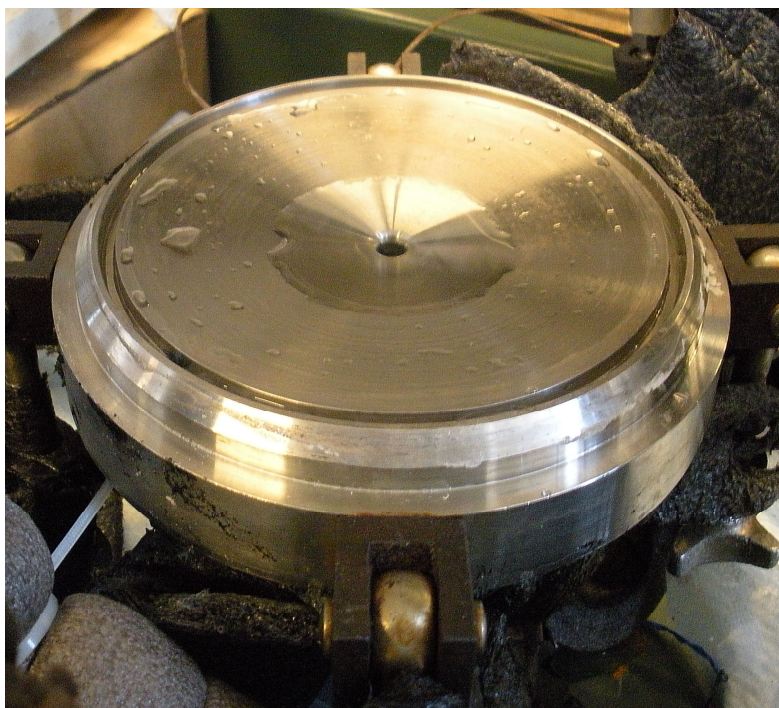
Figure 3.32 Photograph of the brine side of the big cell used for the experiments.
