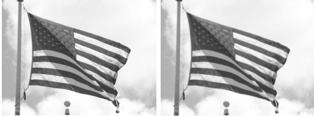
Figure 4.4 Comparison between doubly compressed image and its low-pass filtered image. (left) Doubly compressed image generated from ucid01248 using (QF1, QF2) = (60, 80) ; (right) The anti-forensically modified image generated by convoluting a 3 \times 3 mean filter on the doubly compressed image. PSNR (dB) between two images is 34.57 dB (the left picture was used as a reference image).
