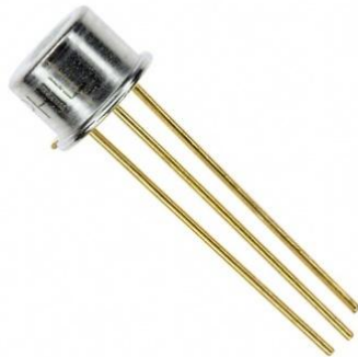
Figure 1.5 AD590 temperature sensor [9]
