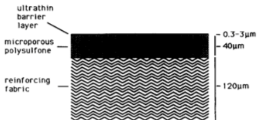
Figure 1.2 Schematic diagram of a thin film composite membrane (Peterson, 1993).
