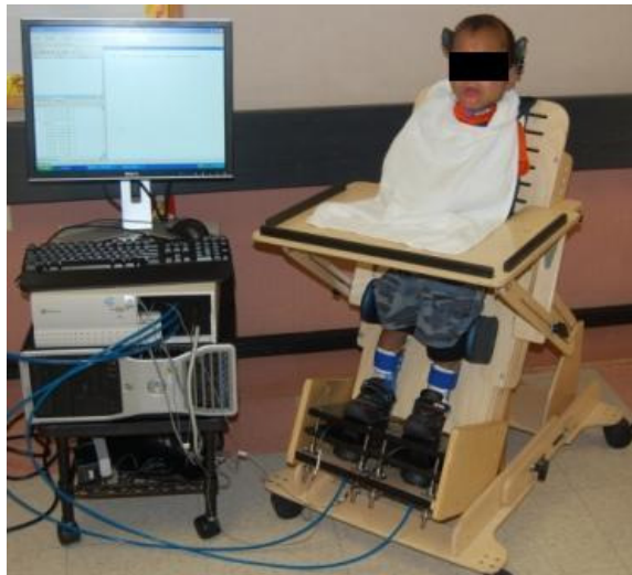
Figure 2.3. Finished set-up of the dynamic standing system. (Not pictured is the hospital grade compressor used to control the pneumatic actuators.)
