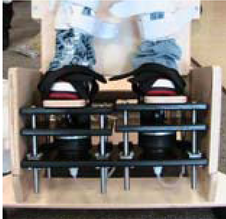
Figure 2.3 Dynamic stander footplate. The dynamic footplate was incorporated into the standing frame of current passive standers to minimize the training required to place and secure the children in the dynamic stander. Pneumatic actuators were used as they are relatively quiet and easily programmed in MATLAB ® . Load cells were placed in between the top and middle plates to allow the forces being applied to the feet to be recorded throughout the study. Mechanical stops were placed on the distal end of the shafts to limit the vertical displacement to one centimeter and minimize the risk of chafing at the straps.
