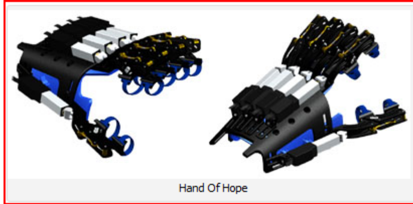
Figure 1.4 The Hand of Hope device combines EMG technology with a robotic exoskeleton to improve hemiparetic finger motion [41].
