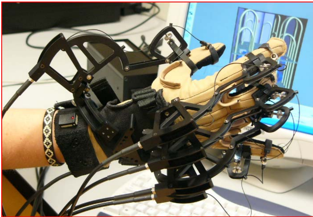
Figure 2.2 The CyberGrasp™ exoskeleton, worn over a CyberGlove® [58].
