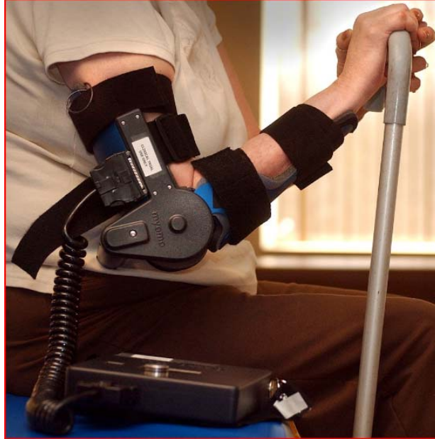
Figure 1.2 The Myomo e100 neurobotic device incorporates EMG technology to improve elbow motion after stroke. After bicep or tricep surface electrodes detect even trace muscle contraction, a motor in the device assists with the individual's desired movement [39].
