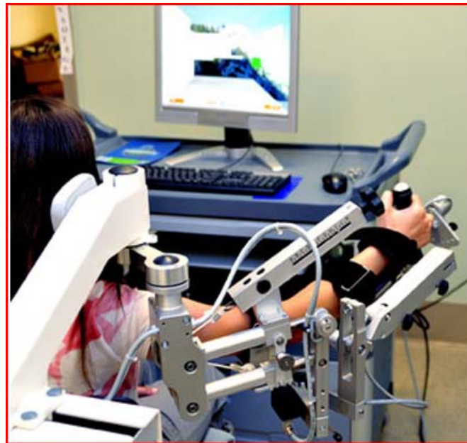
Figure 1.1 A patient engaging in arm exercises in a virtual environment with the Armeo® robotic arm exoskeleton [38].
