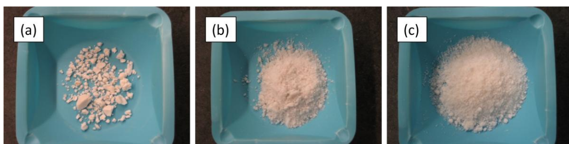
Figure D.3 0.5g of dried nanopowders after stirring in (a) hexane, (b) supercritical CO 2 and (c) liquid CO 2
