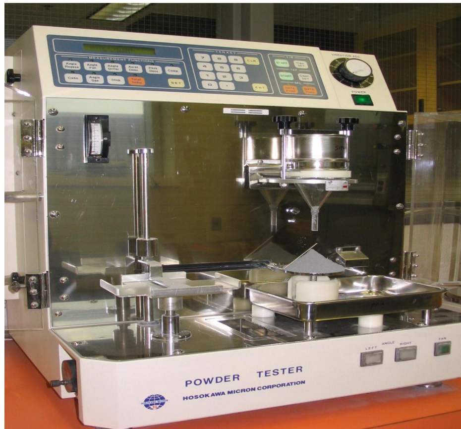
Figure 3.7 Hosokawa Powder Tester set-up.
