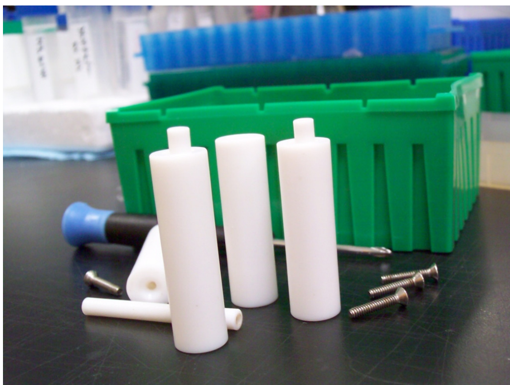
Figure 2.1 The four cylindrical tubes and mandrels used to form the tissue rings.
