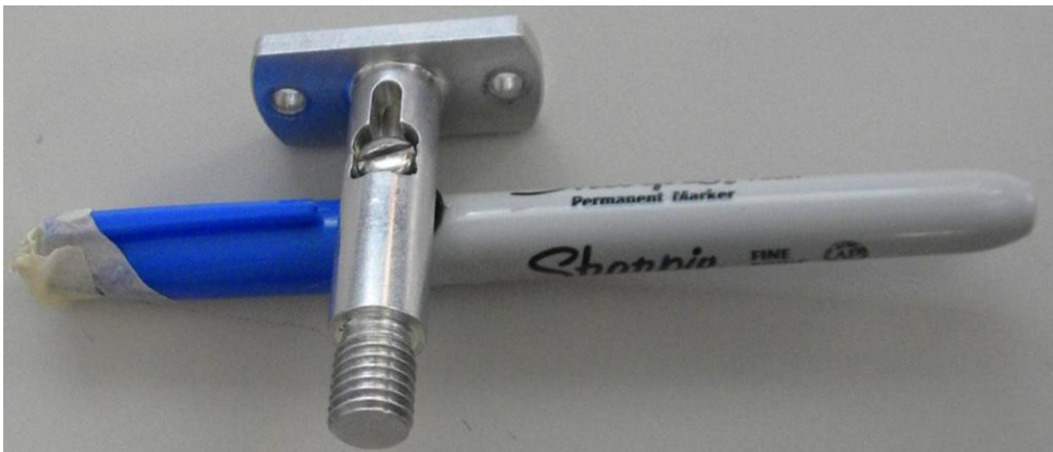
Figure 2.4 Pointer that attaches to haptic master.
