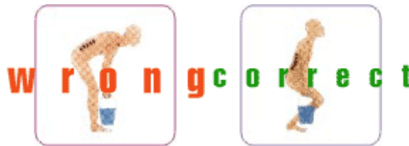
Figure 6.1 (a) Wrong Way of Lifting a Load. (b) Correct Way of Lifting a Load [36]
