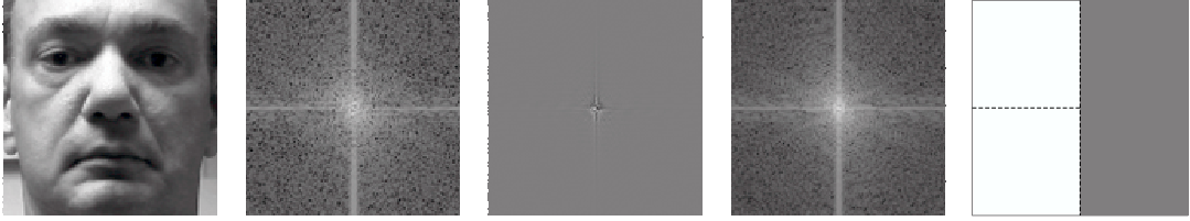
Figure 2.2 The 2D discrete Fourier transform of a face image: the real part (log plot), the imaginary part, and the magnitude (log plot). The frequency features used in the method are extracted from the right two quadrants, as indicated by the gray area.
