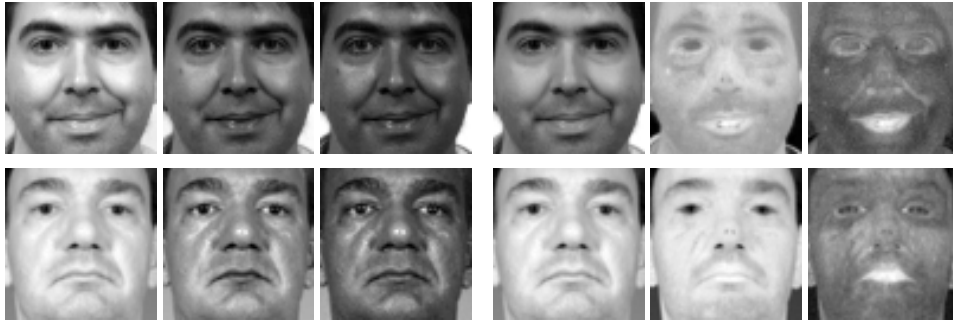
Figure 3.1 Color component images for two subjects in the FERET (top row) and FRGC (bottom row) databases, respectively. From left to right, color component images: R, G, B, V, I, and Q.
