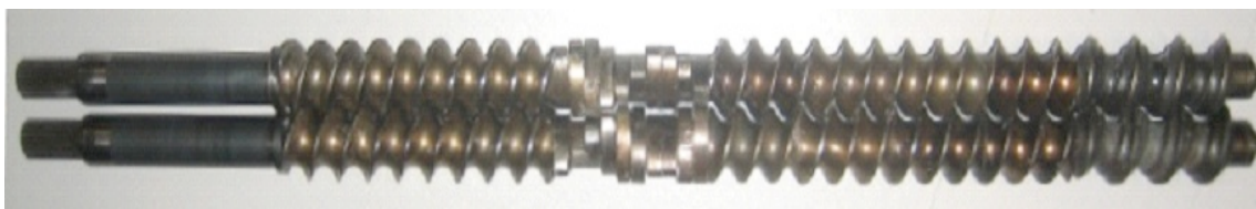
Figure 3.8 Screw configuration of APV twin screw extruder.
