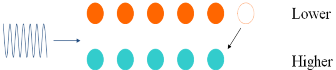
Figure 2.2 Excitation of Spins by RF pulse. Transition of spins from lower energy to higher energy state.
