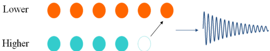
Figure 2.3 Relaxation of Spin System after RF pulse excitation. Transition of spins from higher energy state to lower energy state
