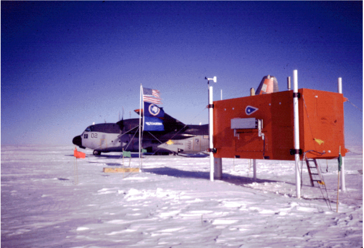
Figure 2.3 An Automated Geophysical Observatory (AGO) in Antarctica. Field engineers are flown to each site about once per year and left for several days as they make various repairs and installations.
