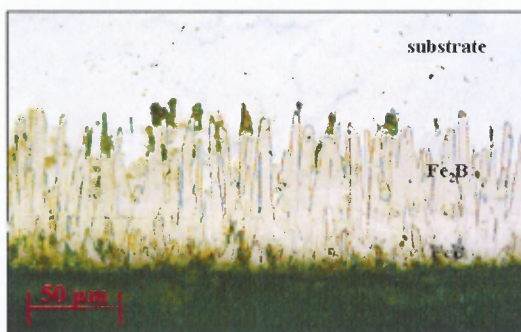
Figure 2.1 The saw-tooth structure of boride layers with the exterior phase of \text{FeB} and the interior phase of \text{Fe}_2\text{B} on AISI 1018.
