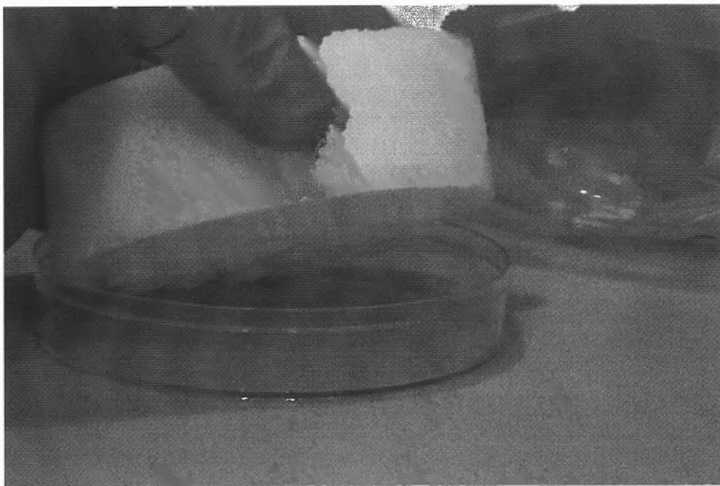
Figure 4.6 Master slowly being placed on the dish to minimize the air trapped inside.
