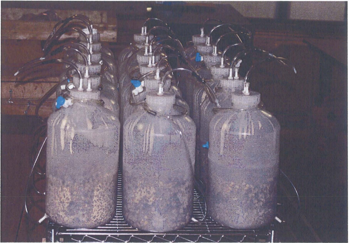
Figure 4.4 Assembled bioreactors used for composition of waste.
