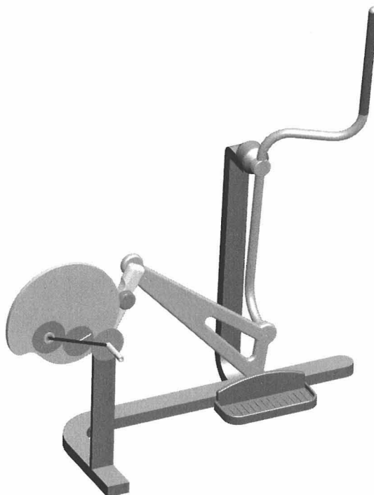
Figure 3.40 3D view of the mechanical timing mechanism added to the four-bar mechanism.
