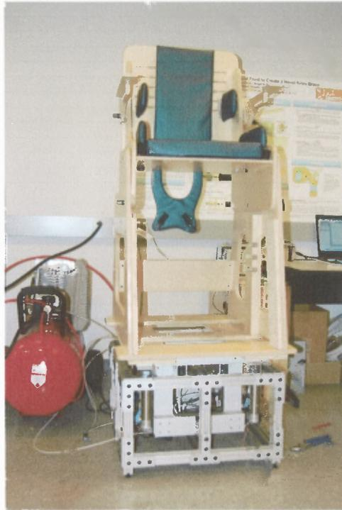
**Figure 4.6** Otolith stimulation device with no additional loading.
