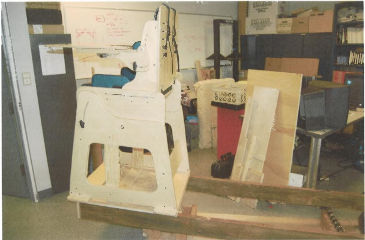
**Figure 2.1** Seesaw otolith stimulation device. Displayed is half of the device, including the chair and fulcrum.
