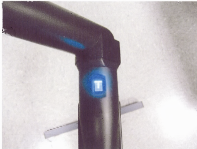
Figure 4.4 The iARM LED display indicates its current status, as well as movement errors or software problems.
