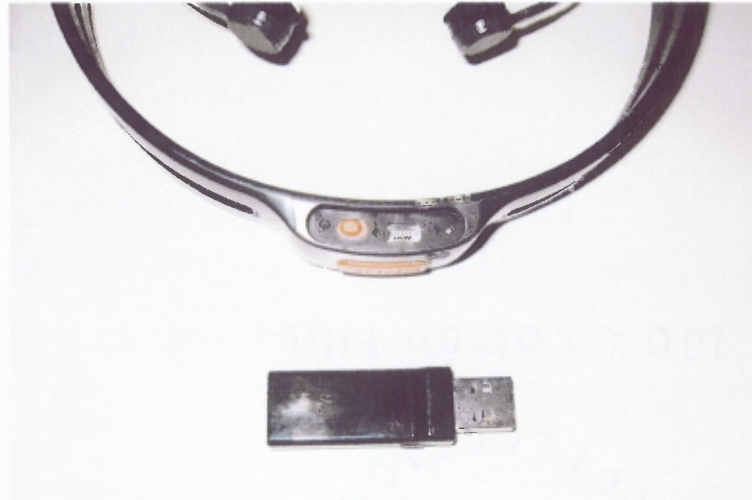
Figure 3.3 The wireless USB connector, power toggle switch and charging socket of the Emotiv EPOC™ are shown here. The toggle switch is currently in the ‘off’ position, whilst sliding it to the USB icon is ‘on’.
