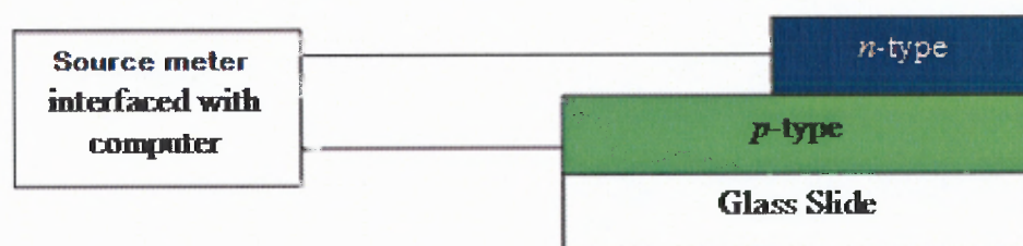
Figure 4.1 Schematic to measure current-voltage characteristics for p - n junction.
