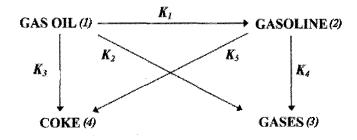
Figure 4.1 Four lumps model for gas oil cracking reactions
