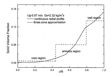
Figure 3.23 Three-zone approximation of inlet condition.
