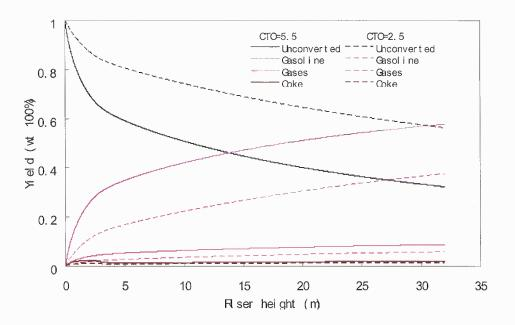
Figure 4.17 Parametrical study of catalyst to oil ratio (5.5 vs. 2.5).
