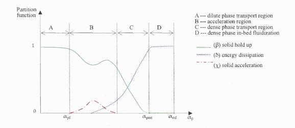
Figure 2.3 General patter of input power partition by  $\beta$ ,  $\delta$ ,  $\chi$  in a riser flow.
