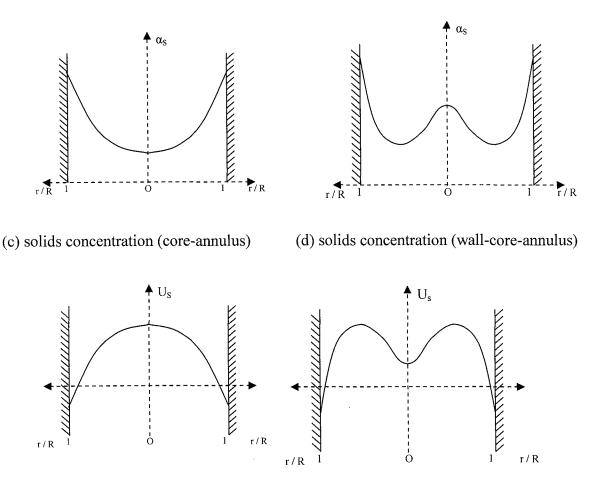
(e) solids velocity (core-annulus)(f) solids velocity (wall-core-annulus)Figure 3.1 Heterogeneous flow structures in risers (in A-A plane) (continued).
