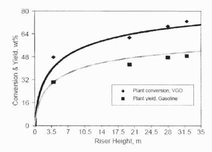
Figure 1.2 Typical conversion & yield pattern of FCC riser.
