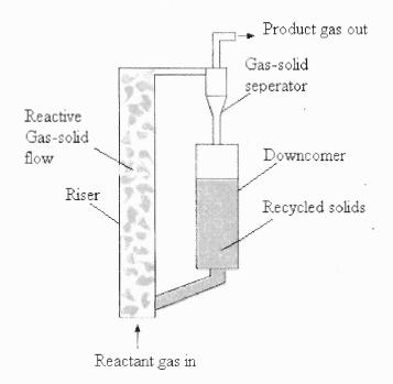
Figure 1.1 Schematic diagram of generic riser configuration.
