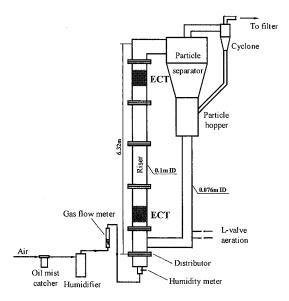
Figure 3.4 Schematic diagram of the riser system (CFB).
