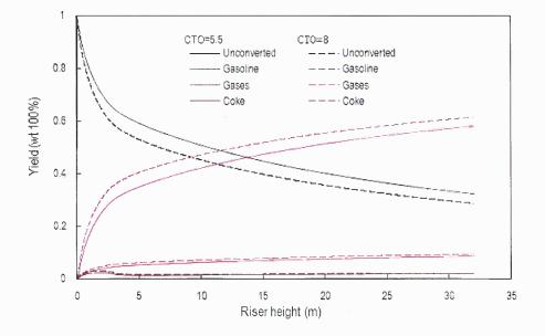
Figure 4.15 Parametrical study of catalyst to oil ratio (5.5 vs. 8.0).
