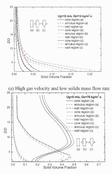
(b) Low gas velocity and high solids mass flow rate Figure 3.26 Parametric study of effects of entrance region.
