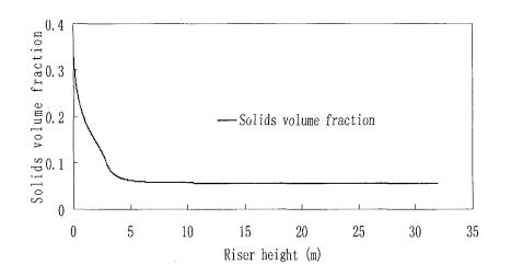
Figure 4.11 Model prediction of solids volume fraction.
