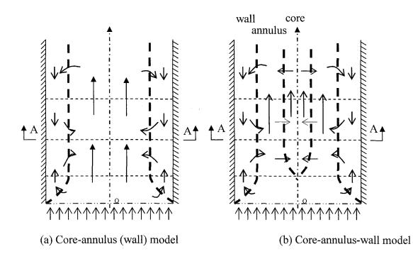
Figure 3.1 Heterogeneous flow structures in risers.
