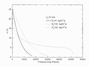
Figure 3.8 Effect of solids mass flow rate on axial pressure distribution.
