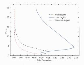
(a) Solid concentration reversal in the core (U=1 m/s).Figure 3.9 Effect of gas inlet velocity on solids concentration structures.
