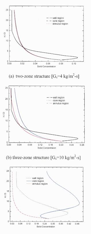
(c) Solid concentration reversal in the core region  $[G_s=50 \text{ kg/m}^2\text{-s}]$ Figure 3.7 Effect of solid mass flow rate on flow structure.
