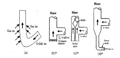
(a) Solids feeding patterns used in the experiment (\* from Du et al. 2004).
