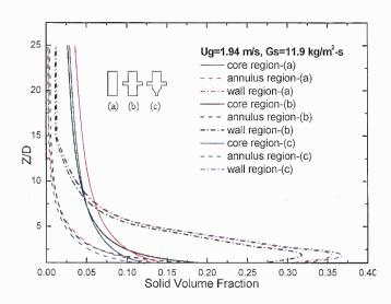
(b) Example of high solids mass flow rate (Ug=1.94m/s, Gs=11.9 kg/m2-s)Figure 3.24 Effect of solids feeding patterns on solids concentration.
