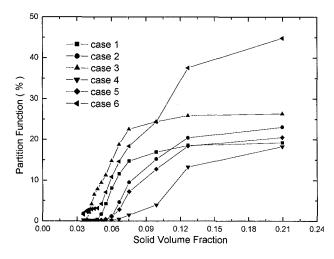
Figure 2.10 Partition function of solid energy dissipation.
