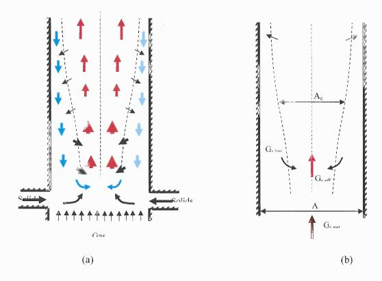
Figure 2.17 Solids flow structure in riser.
