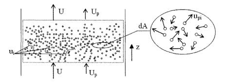
Figure 2.2 Concept of cross-sectional averaged velocities.
