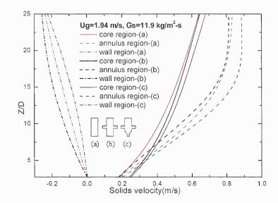
(b) Example of high solids mass flow rate ( $U_g=1.94$ m/s,  $G_s=11.9$  kg/m<sup>2</sup>-s) Figure 3.25 Effect of solids feeding patterns on solids velocity (Continued).
