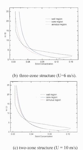
Figure 3.9 Effect of gas inlet velocity on solids concentration structures (Continued).
