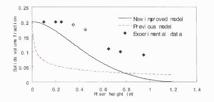
Figure 2.18 Model predictions vs. experimental measurement.
