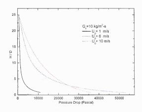
Figure 3.10 Effect of gas velocity on axial distributions of pressure.
