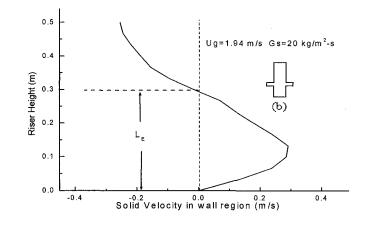
Figure 3.21 Definition of characteristic length of entrance region (L<sub>E</sub>).
