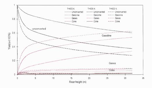
Figure 4.19 Parametrical study of temperature (805K vs. 600K and 900K).
