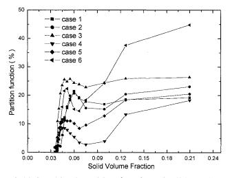
**Figure 2.11** Combined partition function of solid acceleration and energy dissipation.
