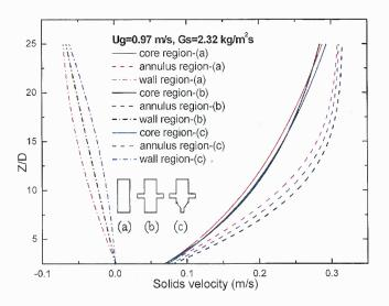
(a) Example of low solids mass flow ( $U_g=0.97$ m/s,  $G_s=2.32$  kg/m<sup>2</sup>-s) Figure 3.25 Effect of solids feeding patterns on solids velocity.
