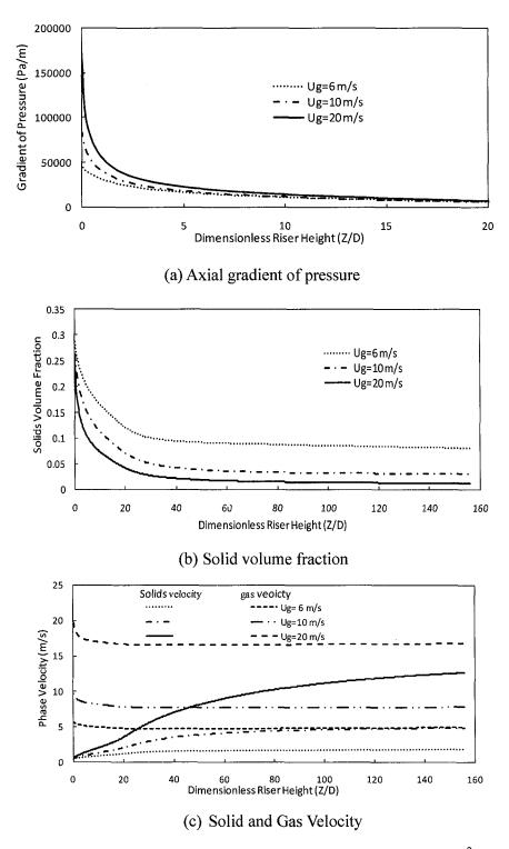
**Figure 2.15** Effect of gas velocity on flow pattern ( $G_s$ = 382 kg/m<sup>2</sup>.s).
