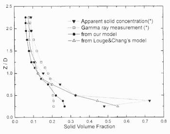
Figure 2.7 Axial solid volume fraction distribution.
