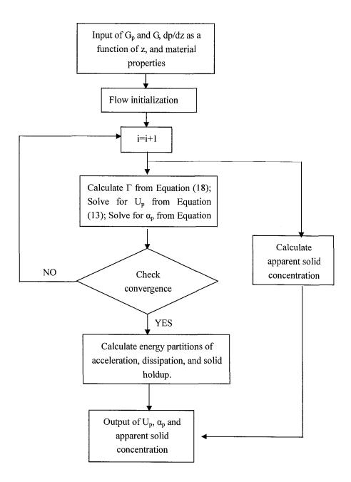
Figure 2.4 Flowchart of model solving procedures.
