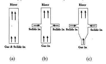
(b) Axial symmetric solids feeding patterns used in 2-D simulations
