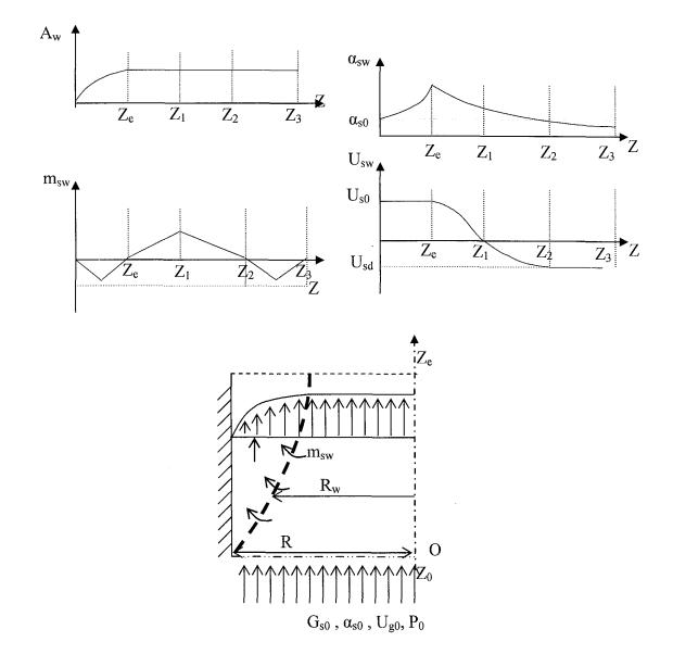
(e) wall-entrance region Figure 3.3 Schematic profiles of solids flow in the wall region.
