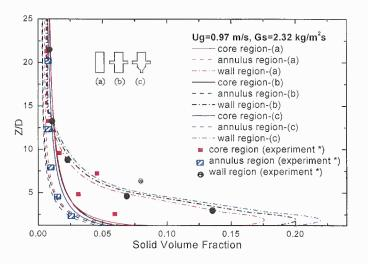
(a) Example of low solids mass flow (Ug=0.97m/s, Gs=2.32 kg/m2-s) (\* data are from Halow JS, et al. 1993)
