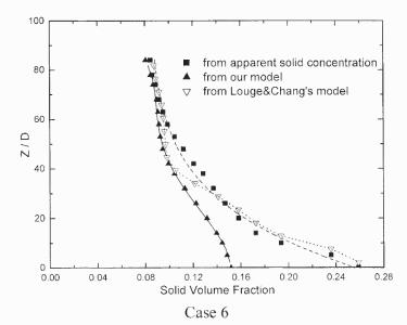
Figure 2.6 Axial solid volume fraction distribution.
