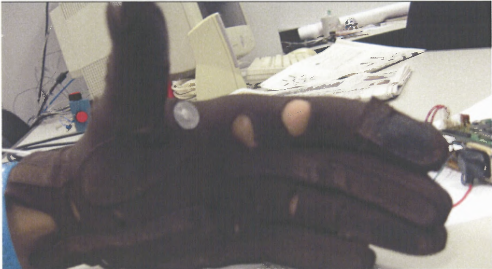
Figure 2.8 Glove with force sensor.
