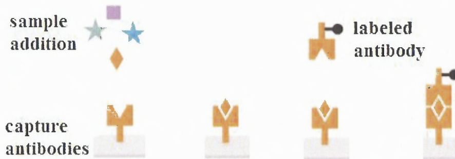
Figure 2.2 Schematic of label-based technique for immunosensing.
