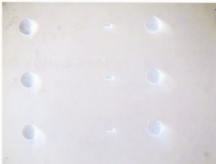
Figure 4.17 Snapshot of the vias taken under the microscope.
