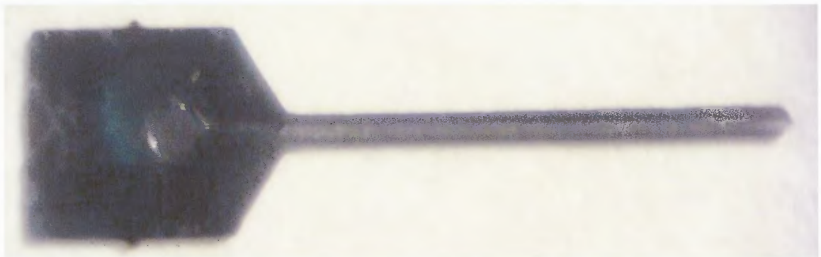
Figure 4.25 Bottom half of microneedle with microchannel seen under microscope.
