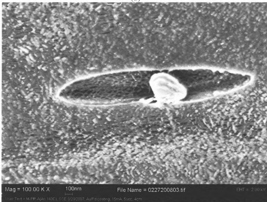
Figure 3.13 SEM images of M-PP(An 140C): (a) spherulitic structure (10000X) (A: radial-like bright region, B: ring-like bright region, C: foreign particle); (b) lamellar opening (100000X), (c) debonding morphology around a foreign particle (100000X).
