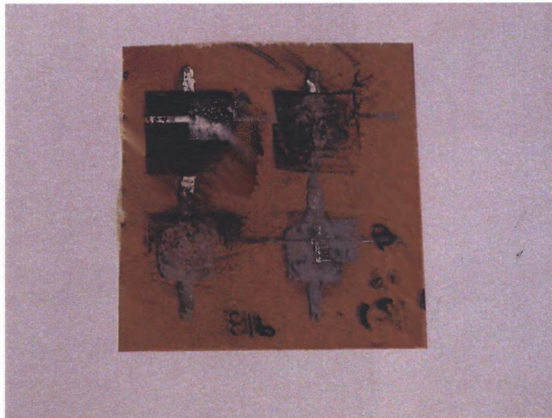
Figure 3.8 Sensor with burned polymer and top contact.
