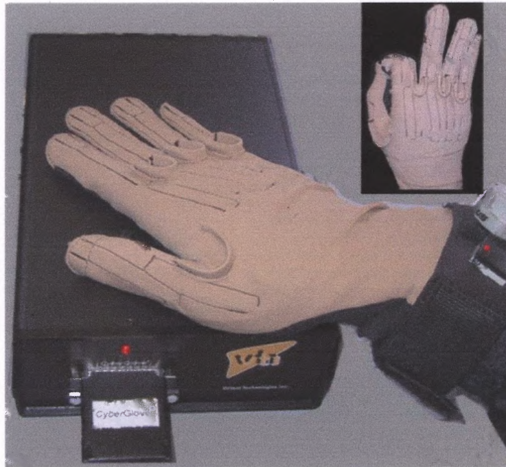
Figure 2.8 Cyber Glove® system for recording finger joint angle data. (Source: http://infolab.usc.edu )
