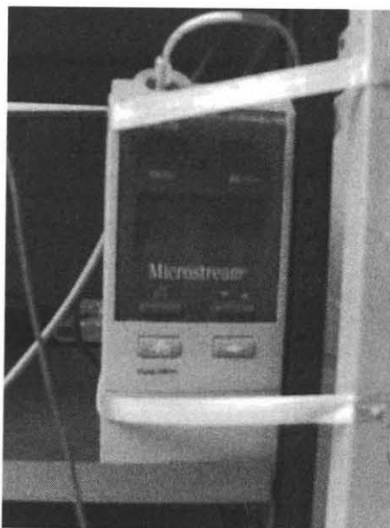
Figure 2.2 End tidal \text{CO}_2 and breath rate monitor used to monitor the animals \text{CO}_2 (model NFB-70, Microstream).
