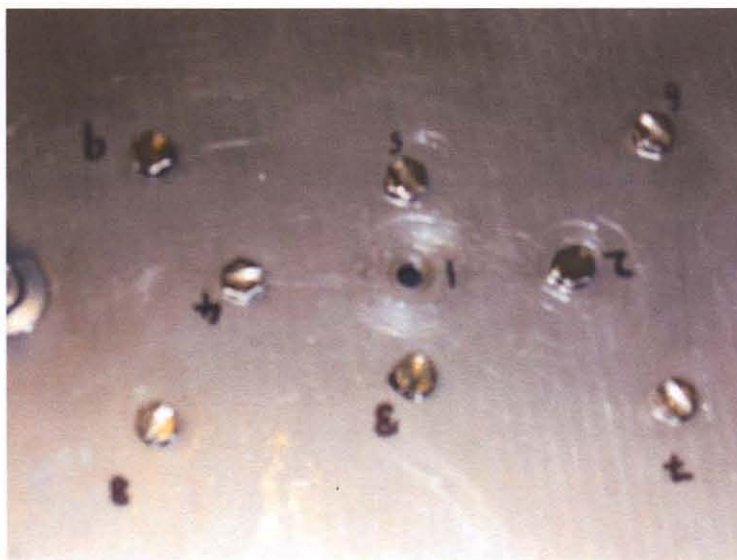
Figure 3.16 Top plate manifold of the multi-well injury apparatus, having 9 points for sensor insertion to test pressure at each location.
