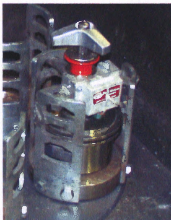
Figure 2.3 Picture of wireless temperature sensor on milling vial.
