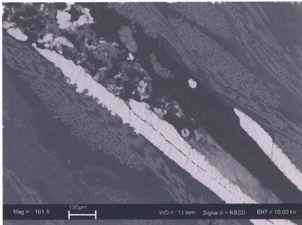
Figure 3.24 Low magnification SEM image showing interface that has some indication of bonding.
