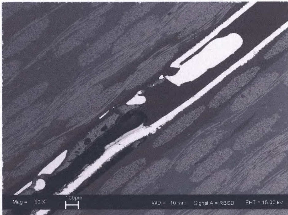
Figure 3.23 Low magnification SEM image of interface for plate which was bonded.
